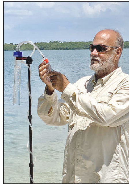
Dr. Manuel Aparicio demonstrating the Calusa Waterkeeper ADAM aerosol sampler
